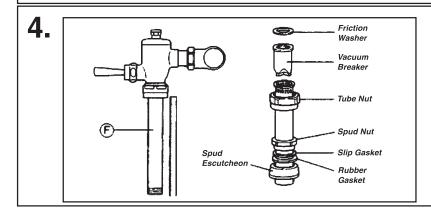
Determine the length of vacuum breaker tube (F) required to join the flushometer valve and fixture spud. Cut the vacuum breaker tube, if required, to this length. Assemble the vacuum breaker tube assembly and spud nut assembly to the flushometer valve and fixture spud.
